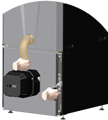
Figure 30 - Checking the installation of the spiro pipe and tightness of the boiler door
